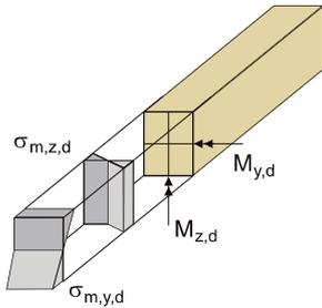
$$k_m \cdot \frac{\sigma_{m,y,d}}{f_{m,y,d}} + \frac{\sigma_{m,z,d}}{f_{m,z,d}} \leq 1$$
