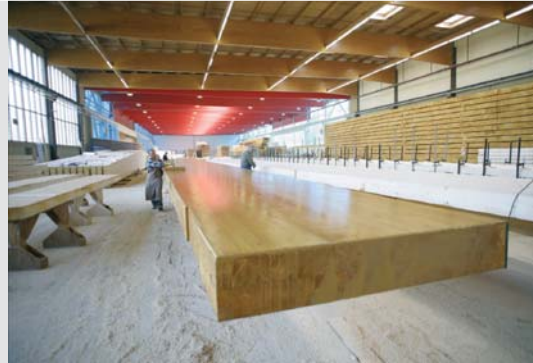
Coating of a glulam beam
