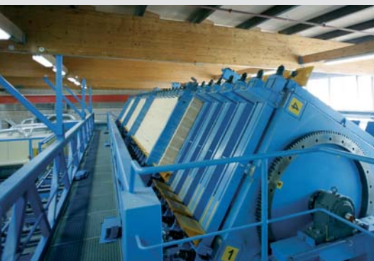
Rotating moulding press, Express-line
